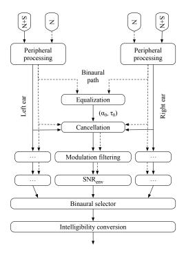
Figure 4.1: Diagram of the model structure. Solid lines denote the path of the speech-plus-noise (S+N) mixture and the dash lines show the path of the noise alone (N). The values  $\alpha_0$  and  $\tau_0$  represent the optimal parameters selected by the equalization process.
