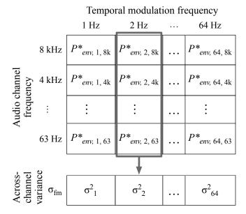
Figure 2.3: Illustration of the calculation of the across-channel variance of the envelope power for a given time frame. Each cell represents the normalized envelope power,  $P^*_{\text{env},g,l}$ , of the noisy speech at the output of a temporal modulation filter g, and audio filter, l. The across-channel variance,  $\sigma_g^2$ , for a given modulation filter center frequency corresponds to the variance across rows for a given column of the matrix.
