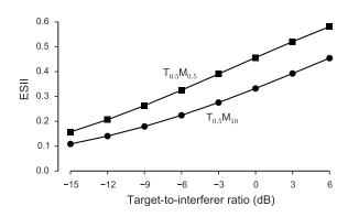
Figure 3.2: ESII prediction for two speech maskers when they are either co-located with the target, at 0.5 m from the listener, or placed 10 m away, on axis.
