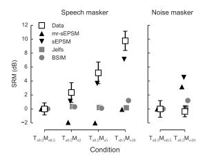
Figure 3.1: Measured SRMs and model SRMs as a function of the masker distance for speech maskers (left) and SMSSN (right). Vertical bars represent one standard deviation.
